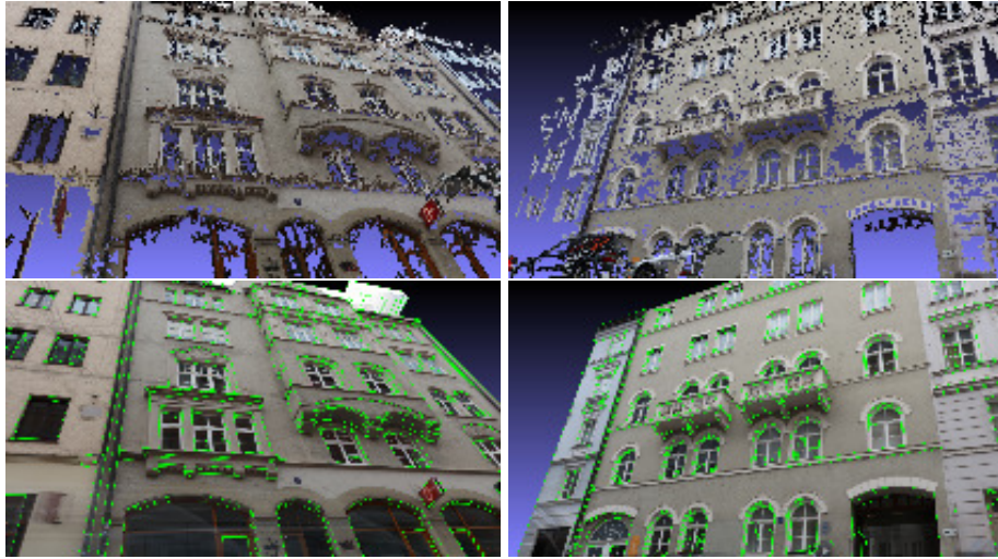
Fig. 11. Top: Input point cloud. Bottom: Textured mesh with highlighted seams.
